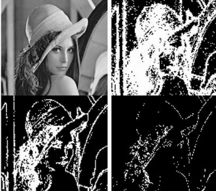
Fig. 4. Regions having entropy more than k threshold: (a) top-left: original image, (b) top-right: k=1 , (c) bottom-left: k=2 and (d) bottom-right: k=3
